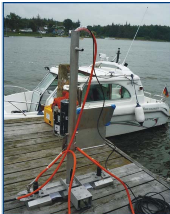
Fig. 2 Multi-transducer parametric echosounder system (©Innomar)
