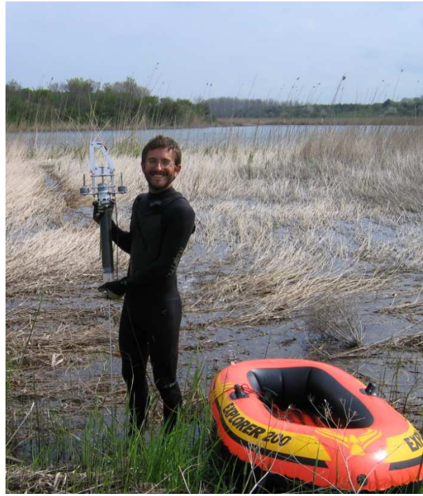
Fig. 2 Small gravity hand corer ('Kajak corer') used for intertidal sites. Lead weights can be added to increase penetration and the corer mechanism closes when the attached rope goes slack. The corer works very well in muddy sediments but less well in sandy sediments. © S. Gabriel
