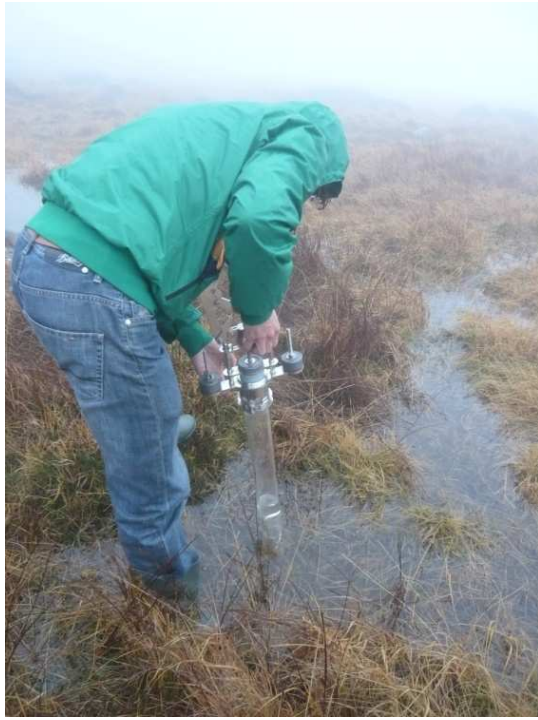
Fig. 2 Small gravity hand corer ('Kajak corer') used for intertidal sites. Lead weights can be added to increase penetration and the corer mechanism closes when the attached rope goes slack. The corer works very well in muddy sediments but less well in sandy sediments. © S. Gabriel
