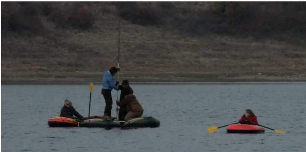
Fig. 3 Manual piston corer ('Livingstone core sampler') used on a small lake. The corer works well in soft sediments but is less adapted to more compact clays or sandy sediments. . © S. Gabriel
