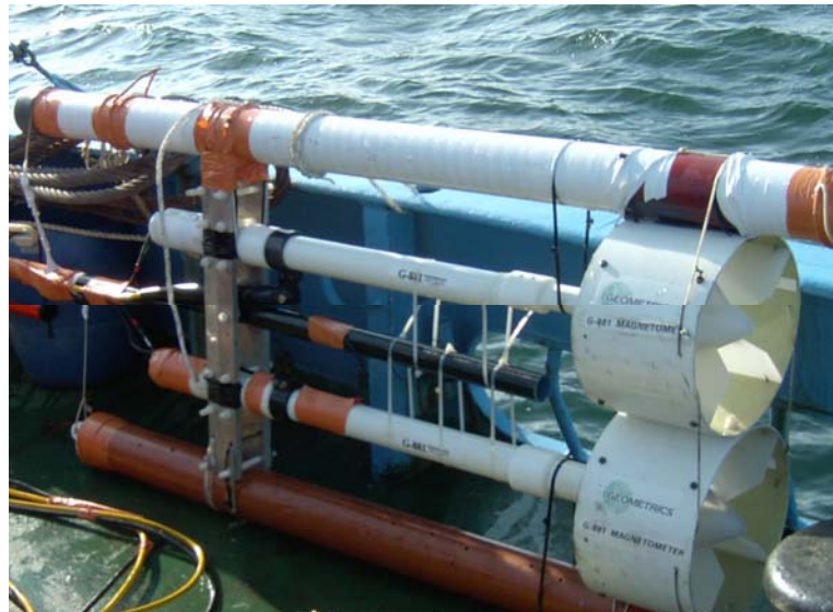
Fig. 2 Marine magnetometer array in vertical gradient acquisition mode (©G-Tec)
