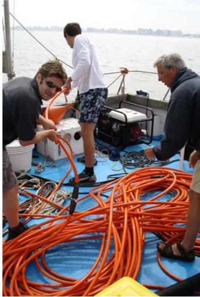
*Fig. 1 Deployment of bottom electric cable for marine resistivity survey (© RCMG Universiteit Gent)*
