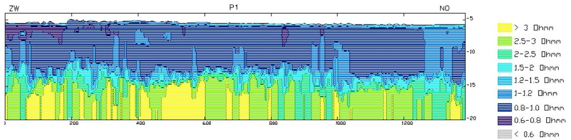
Fig. 4 2D resistivity section off the Belgian coast showing a succession of sandy and silty sediments (© RCMG Universiteit Gent).
