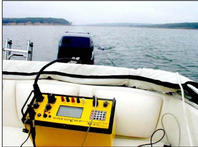
Fig. 3 Marine resistivity acquisition unit (© AGI Super Sting)
