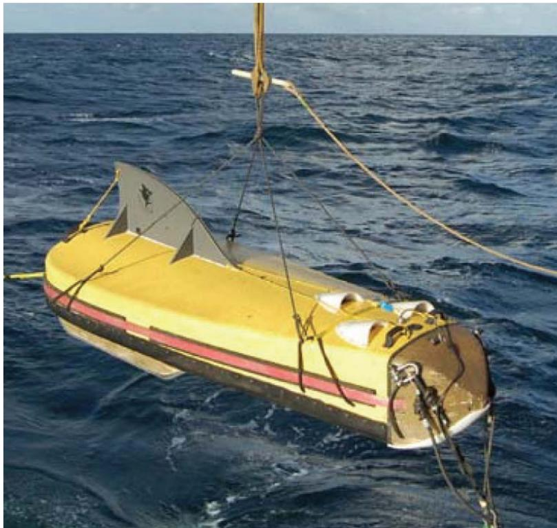
*Fig. 2 Bottom-towed EM profiler array "GEM-Shark" for marine surveys
