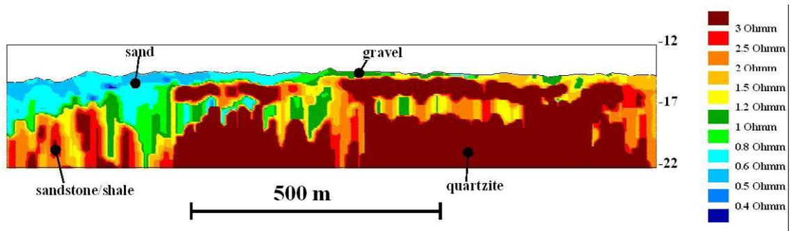
Fig. 5 2D resistivity section recorded offshore Spain showing a harder structure overlying softer sediments (© DEMCO).
