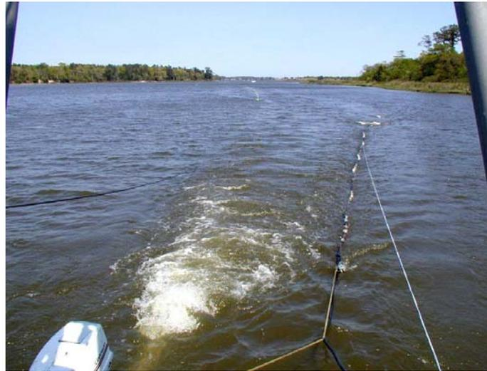
*Fig. 2 Floating electrode cable during marine resistivity survey (© AGI)*
