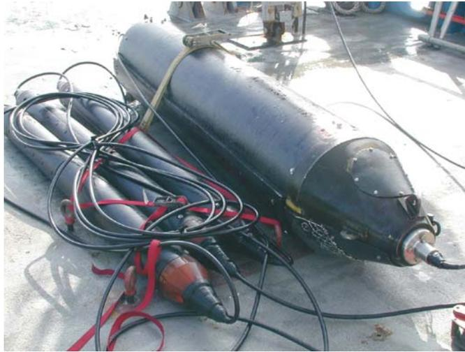
*Fig. 1. FEM profiler array for marine surveys. Left: receivers, right: source
