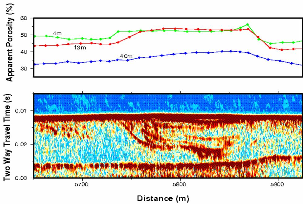
Fig. 3 Porosity profile (top) and concurrent acoustic) recorded offshore North Carolina (© WHOI)
